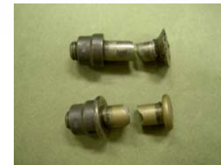
1/4-Inch Diameter Titanium Hex-Drive Fasteners with CRES Tension Collars, Ti-CFRP-Ti Stacks, t/d = 2.1–2.7
